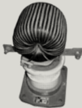
Abb. 16 Stromwandler A20P1, SSW, 1925
